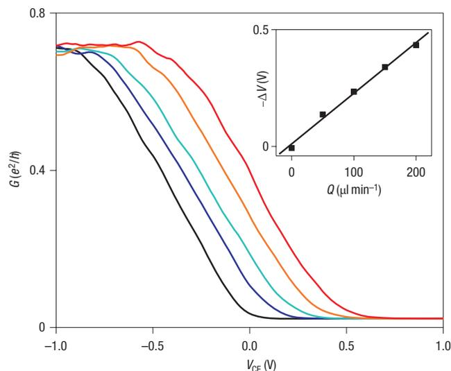
**Figure 2** Shift in nanotube transistor threshold voltage with liquid flow rate. Conductance versus counter-electrode voltage for different flow rates (the black, blue, light blue, orange and red curves correspond, respectively, to flow rates of 0, 50, 100, 150 and  $200 \mu\text{l min}^{-1}$ ). The inset shows threshold voltage versus flow rate. The data closely follow a linear trend.
