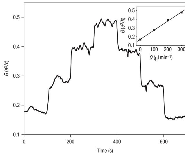
**Figure 4** Flow sensor operation. Conductance versus time for a semiconducting nanotube device as the flow rate is stepped up sequentially through 0, 100, 200 and  $300 \mu\text{l min}^{-1}$ , and then back down sequentially through the same values.  $V_{CE}$  is held constant at  $-0.2$  V. The inset shows nanotube conductance versus flow rate, in which the device acts as a flow sensor.
