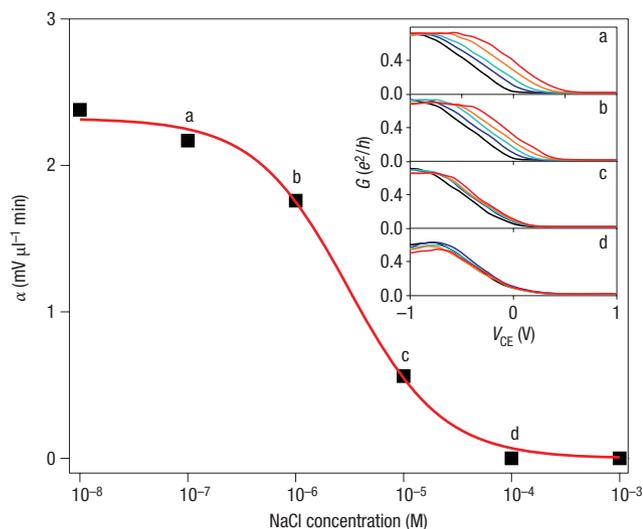
**Figure 3** Nanotube transistor threshold shift for different ionic concentrations. Parameter  $\alpha$  (slope of threshold voltage versus flow rate) versus NaCl concentration. The inset shows conductance versus counter-electrode voltage data, where a–d indicate concentrations according to the points a–d in the main panel from which  $\alpha$  was extracted.
