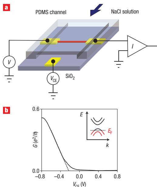
**Figure 1** Experimental setup for the nanotube-based flow sensor and nanotube transistor conductance versus counter-electrode voltage.
