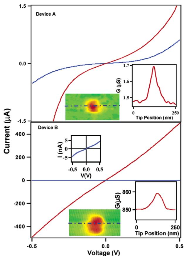
**Figure 3.**  $I$ – $V$  characteristics of two different devices in their “off” (blue) and “on” (red) states, respectively (upper left inset for device B shows the  $I$ – $V$  of the “off” state with an expanded scale). The insets in the lower-right quadrants show the color images of local conductance peaks at high magnification (color scale denotes conductance) and the line traces along the dotted lines.
